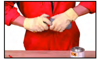
Chamfering the pipe
